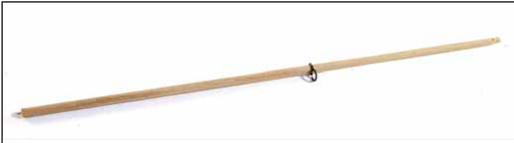
295. Take the last section of dowel and shape as per plan and fit the PE part as per plan. Please note that I added another small length of brass wire to the end of this dowel.
