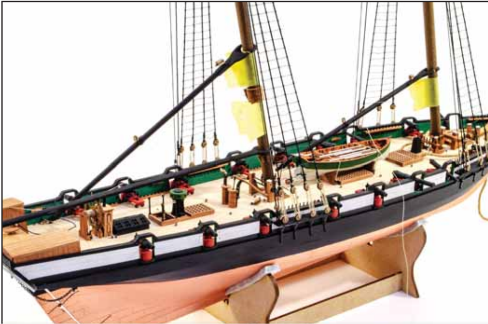
324. At this point, you should look at fitting the gaff/boom assemblies to the masts, simple because the access is easier at this point. The tape you can see is to hold the assemblies in rough place while adding the parrel beads etc.
