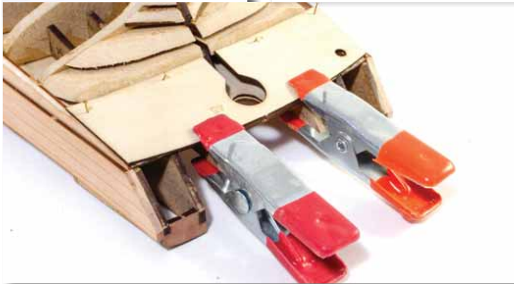
94. Here you can see the plank glued, fitted, and pinned. It's important to also edge glue these planks to each other as well as to the bulkheads. You'll also see that I've only added the plank up to the set of double bulkheads. This is fine as you can fit this first layer in halves, if you wish.
