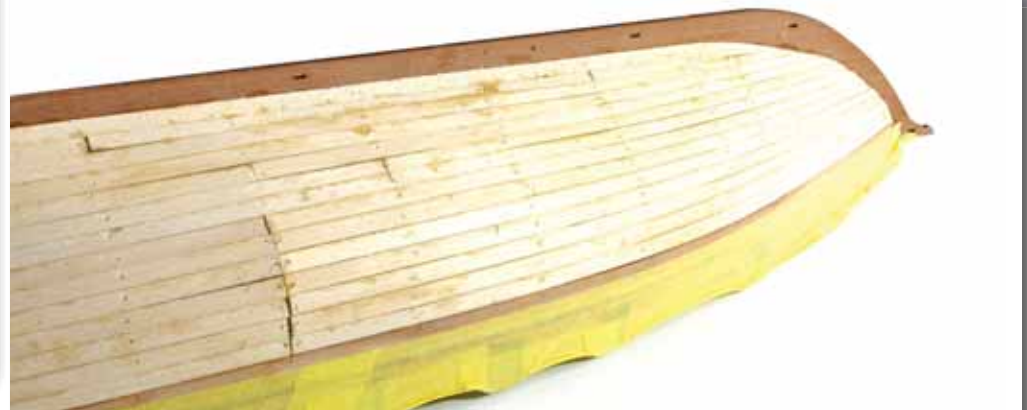
96. Continue to plank the hull, tapering as you go. You will find it beneficial to start tapering the planks from around the double bulkhead point as you progress. No tapering needs to be done at the stern.
