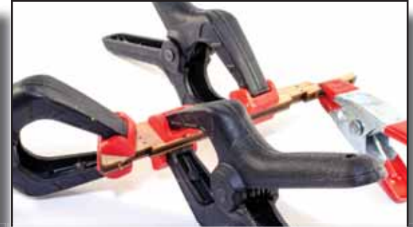
148. Glue the 1mm parts to either side of the 2mm part, ensuring the engraved sides are on the outside.
