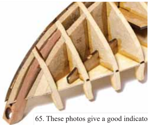
64. Before you can plank the hull, it needs to be prepared. This process of sanding the frames is called 'fairing'. Sand the bulkheads so that the shape of the frames 'flows' and sitting a plank along its length will show a maximum contact area between plank and bulkhead. A good indicator that you are fairing correctly is when most/all of the bulkhead char is gone. Use a sanding stick or similar to fair the hull.
