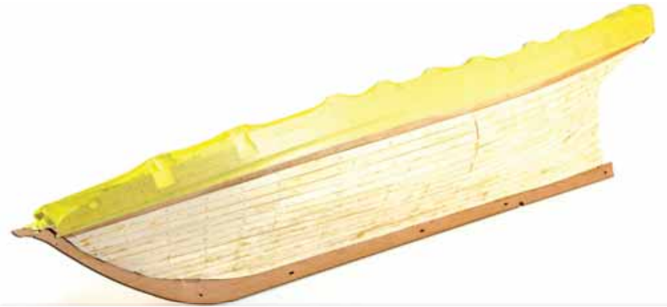
97. The hull is now fully planked. Use scrap planks to fill in any gaps you may have at the stern (or anywhere!).
