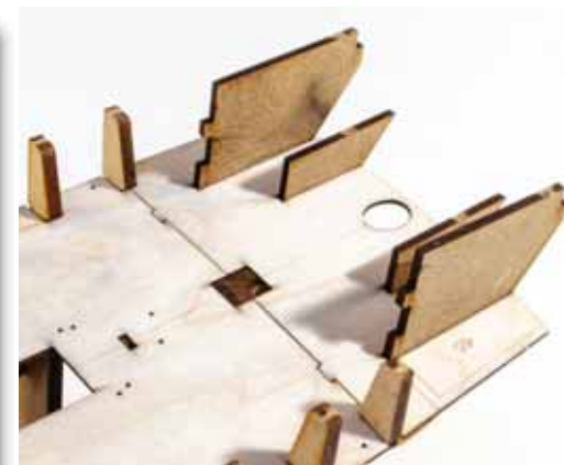
52. Slot the part into place as shown. The front edge will also clip into the bulkhead ears as per the previous deck section.
