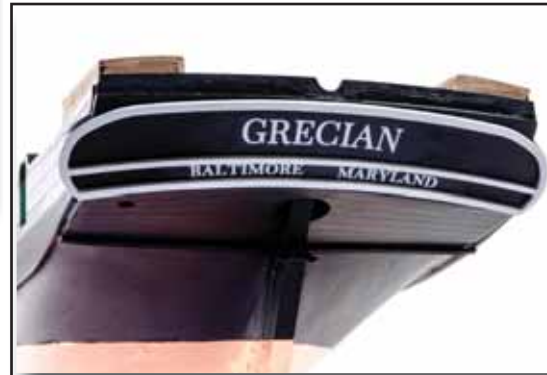
164. This can now be painted white and fitted to the stern as shown. Use the decal sheet to add the details as shown. We have supplied options for you in terms of colour and home port decal. We suggest the decals are added to the surface once it has been glossed. This will provide better adhesion.
