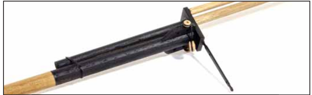
298. Paint this section in black and fit the thimbles and deadeye as shown on plan.
