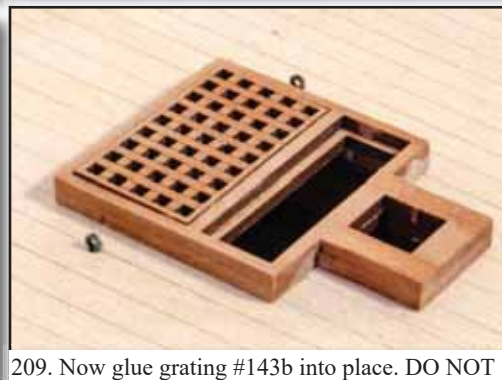
209. Now glue grating #143b into place. DO NOT glue #143c at this point.
