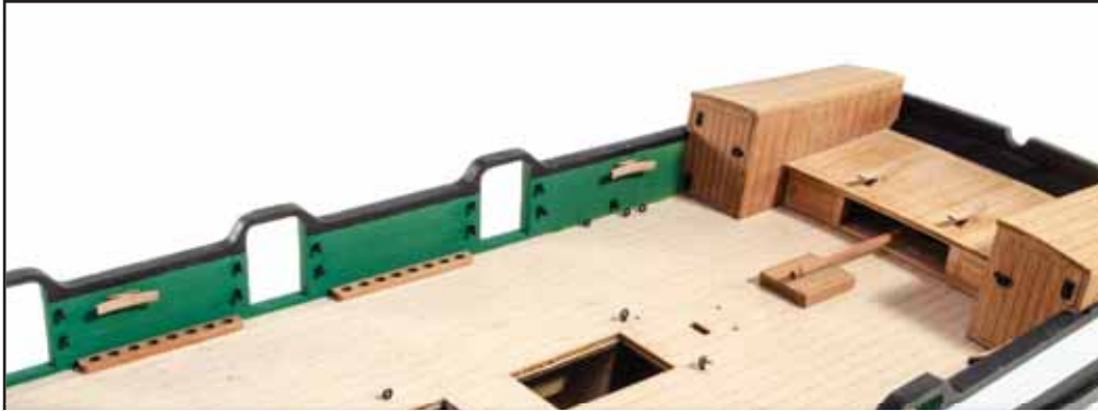
175. From the 1.5mm wood sheet, remove the cleats, part #150, and glue into position as shown here and on plan, not forgetting the two on the small rudder tiller roof at the stern.
