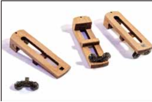
250. Take a set of 3D printed carronade wheels F-4 and glue into place. Sand flush the upper side where the part protrudes through.
