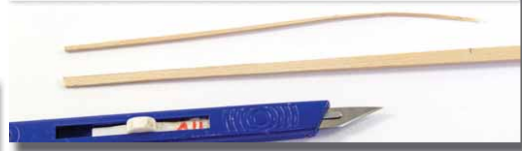
93. Now cut along that line as shown. You will also need to angle the front of the plank to match the curve of the prow, and angle its inner face so it will meet the prow properly.
