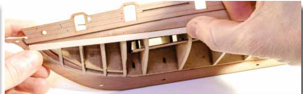
91. We can now begin to add the first layer of planks. You will need to start tapering these from laying the very first one due to how shallow the bow is in relation to the stern. Lie your plank under the bulwark as shown and make a pencil mark where the plank tries to cross over the bulwark.
