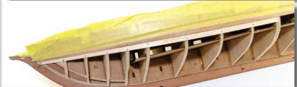
94. Here you can see the plank glued, fitted, and pinned. It's important to also edge glue these planks to each other as well as to the bulkheads. You'll also see that I've only added the plank up to the set of double bulkheads. This is fine as you can fit this first layer in halves, if you wish.
